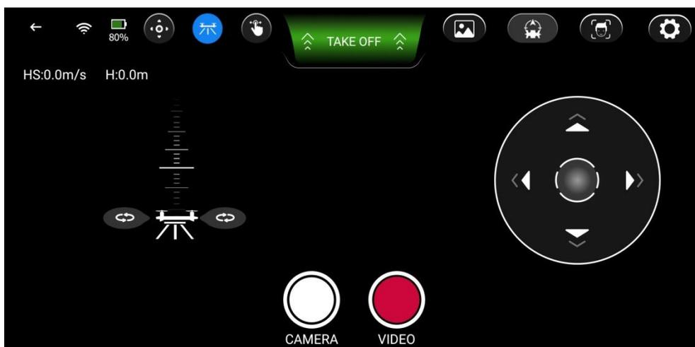
Control SELFLY as if you are controlling a camera mounted on a tripod. On the left you have an icon of SELFLY on a tripod, you can set the height by moving the SELFLY icon up and down on the scale. To rotate left and right press the two arrows on the sides, each time you press the arrow SELFLY will rotate by 20 °-30° accordingly. The right stick is normal pitch (up/down) and roll (left/right).
